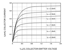
Figure 1. Static Characteristic
