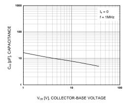
Figure 5. Collector Output Capacitance
