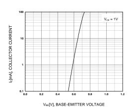
Figure 4. Base-Emitter On Voltage
