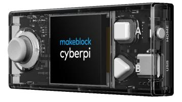
Mounted on the mBot2 there is a CyberPi. A CyberPi is a small, programmable microcomputer. You give the CyberPi commands using the code blocks in mBlock. The CyberPi passes these commands back to the mBot2. You can remove the CyberPi from the mBot2.
