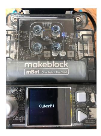
You can display the data from the sensors in different ways on the display of the mBot2. You can use different code blocks for this. These code blocks can be found in mBlock under the category 'Display'.
