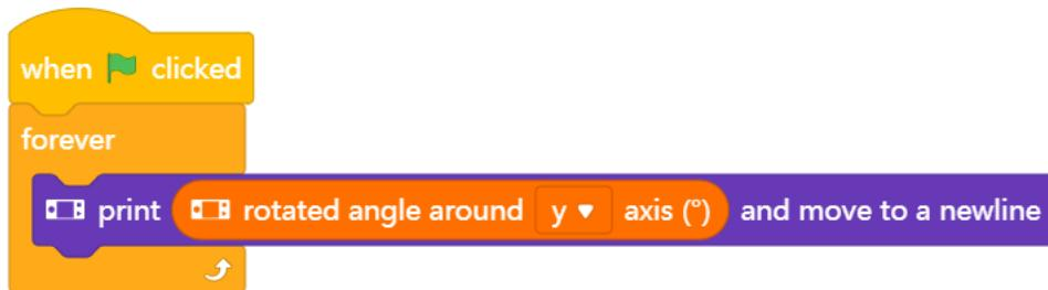
There are two important aspects: this block will keep track of rotational movements that are greater than one revolution. Use this block to count how many times the robot has turned. Looking at the z-Axis, a clockwise rotation will increase the values reported by this block:
