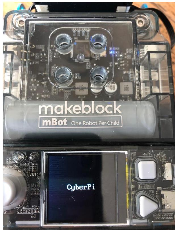
You can display the data from the sensors in different ways on the display of the mBot2. You can use different code blocks for this. These code blocks can be found in mBlock under the category 'Display'.
