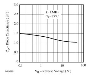
Figure 4. Diode Capacitance vs. Reverse Voltage
