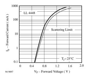
Figure 2. Forward Current vs. Forward Voltage
