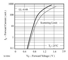
Figure 1. Forward Current vs. Forward Voltage
