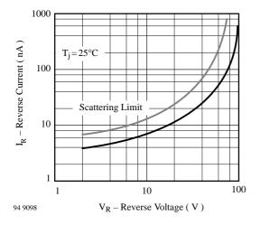
Figure 3. Reverse Current vs. Reverse Voltage
