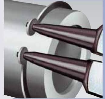
Easy fitting of external circlips
