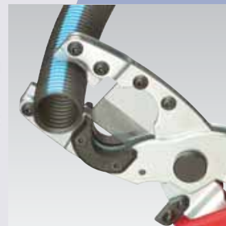
Clean cut of protective tubes 18 – 35 mm dia.
