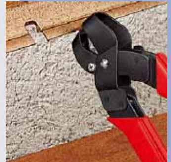
Easy notching thanks to high leverage
