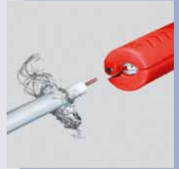
Stripping the conductor of a Coax-cable
