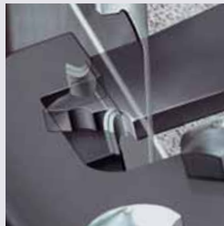
The sheet projections are bent
