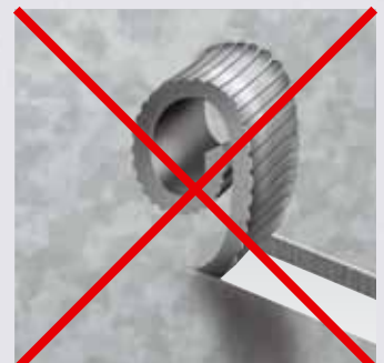
Notching without chip breaking
