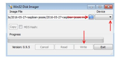
Once the process is complete, you can insert the micro-SD card into your Raspberry Pi and start it.
