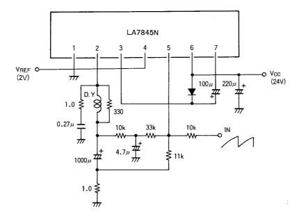
Unit (resistance:  $\Omega$ , capacitance: F)
