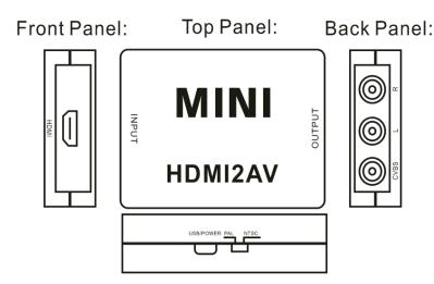
HDMI------HDMI signal input USB POWER------USB power input PAL/NTSC-----PAL/NTSC switch CVBS-----CVBS output L/R-----Audio output
