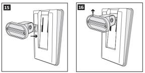
ATTENTION: Ensure that the holder is properly fixed into the device, otherwise it will prevent from using the back tamper switch for supervision of the enclosure's back side. If you do not wish to use the back tamper switch still, please disable it by setting a jumper on DIS-TAMP2 pins (see 2.2. Main Unit and LED Functionality).
