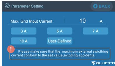
**Note:** The Grid Input Current is set at 10A by default. The change only takes effect when EP500Pro connects to the grid.
