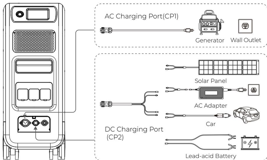
EP500Pro also supports dual charging via AC input and DC1/DC2 input ports simultaneously.
