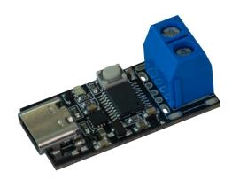
With this small module, you can trigger USB-PD protocols and thus, for example, charge your laptop via a PD-capable USB-C power supply. The output voltage can be adjusted in 5 steps (5 V, 9 V, 12 V, 15 V and 20 V) via the button integrated on the module. The currently selected voltage can be read from the colour of the RGB LED integrated on the module. The module can be used flexibly and is highly integrable.
