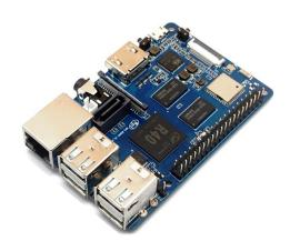
The new Banana Pi M2 Berry is identically constructed as the Raspberry Pi 3B and completely compatible to all the Raspberry accessory.
