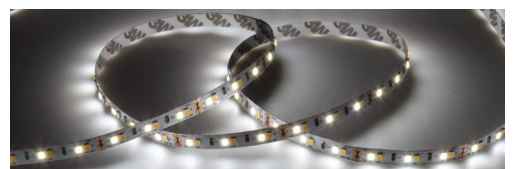
Index: R-2835-600-20-BIK-02 PREMIUM BICOLOR LED strip type 2835, IP20, 120 LED/m, 8-mm width, 6 pts/5 cm, 5-metre roll, power of 10W/m, 1100 lm/m EAN code: 5900652141531
