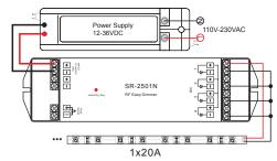
2)Receiver Connection Diagram for Multiple Units
