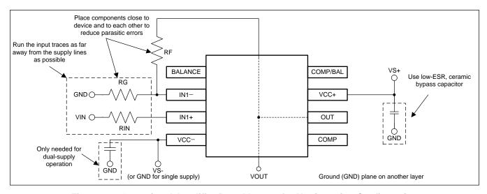
Figure 16. Operational Amplifier Board Layout for Noninverting Configuration
