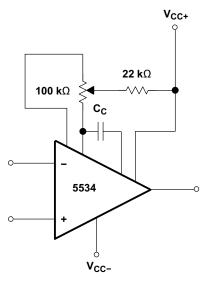
Frequency Compensation and Offset-Voltage Nulling Circuit
