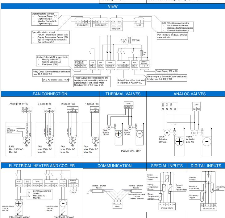
4 · Note, an incorrect wiring of this product can damage it and lead to other hazards. Make sure the product has been correctly wired before turning the power ON.
