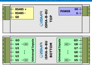
All GO terminals are connected together internally
