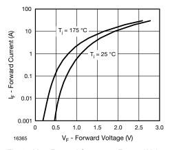
Fig. 2 - Max. Forward Current vs. Forward Voltage
