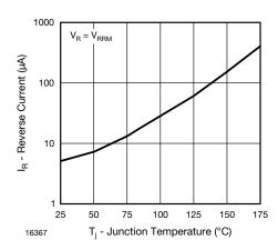
Fig. 4 - Max. Reverse Current vs. Junction Temperature
