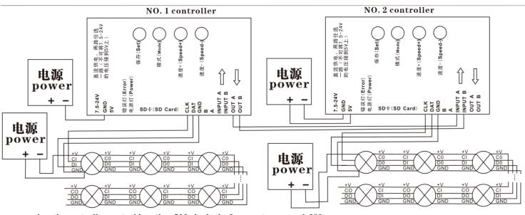
when the controller control less than 512 pixels the frame rate can reach 30 fps, when control more than 512 pixels the frame rate will slow down automatically.
