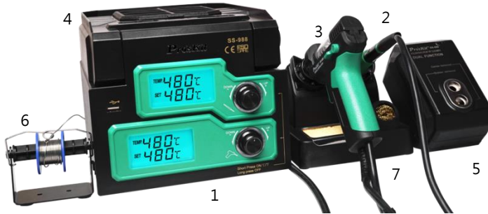
1. Soldering / desoldering station 2.Soldering iron 3.Desoldering gun 4.Smoke absorber & LED light 5. Soldering iron tip cleaner 6.Soldering wire stand 7. Soldering iron stand
