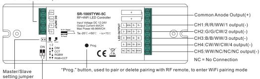
Dial switch for device mode selection, DIM, CCT, RGBW and RGB+CCT 4 modes are available, factory default is RGB+CCT mode
