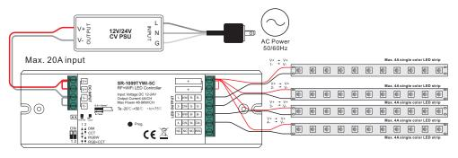
Note: please make sure the dip switches are at position for DIM mode as shown in above diagram.
