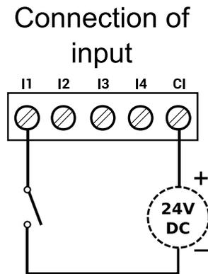
Picture 5 – Connection of input
