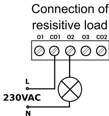
Picture 6 – Connection of resistive load
