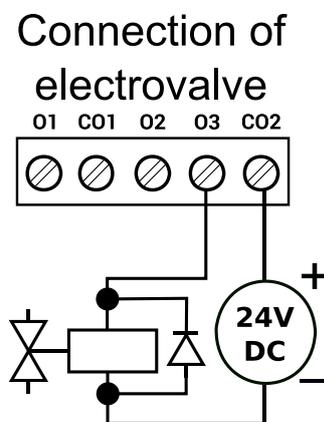
Picture 7 – Connection of electrovalve
