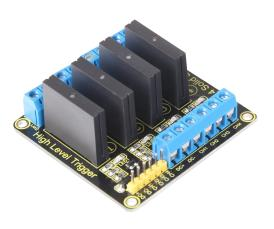
This 4-channel semiconductor relay is suitable for switching alternating current. It has a galvanic isolation by integrated optocouplers and the switching of the load is done with transistors, which is why it has a much longer lifetime than mechanical relays.
