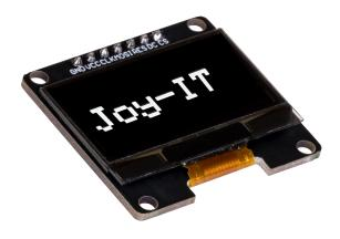
This graphical 1.3" OLED display has a resolution of 128 x 64 pixels and communicates via the SPI interface. Optionally, the display can also be soldered to the I2C interface on the back. This makes the display particularly universally applicable.
