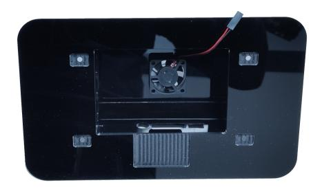
The fan is screwed from the outside with the long black screws.
