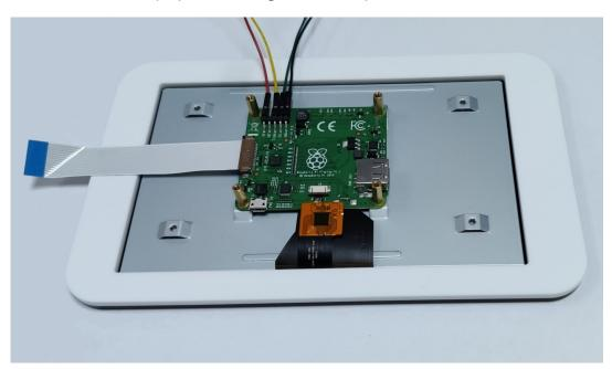
3. Screw the Raspberry Pi 4 onto the spacers of the display board after all cable are placed on the display.
