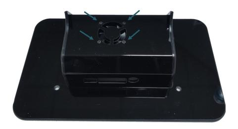
6. Connect the fan to the Raspberry Pi.
