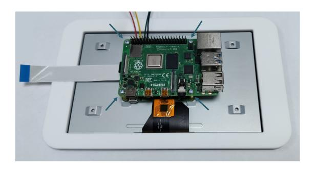
Connect the cables to the Raspberry Pi 4.
