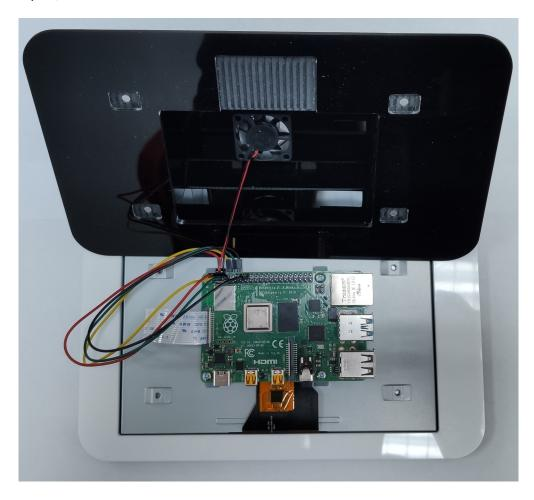
7. Finally, screw the back of the case to the display.
