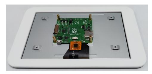
2. Now connect the cables which are in the scope of delievery of the display, to the display board. Make sure that the display cable is aligned correctly.
