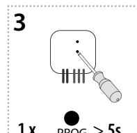
Press of programming button longer than 5 seconds, will activate actuator into timing mode. LED flashes 2x in each 1s interval. After releasing the button, the time of the sunrise function begins to count down (period of complete illumination of the light).
