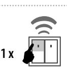
After pressing the programmed button, the light begins to dim in the programmed time interval in a range of 2 seconds to 30 minutes.
