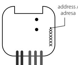
The address listed on the front of the actuator is used for programming and controlling actuators by RF control units.
