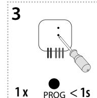
Press of programming button on actuator RFDAC-71B shorter then 1 second will finish programming mode. The LED lights up according to the pre-set memory function.
