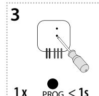
Press of programming button on actuator RFDAC-71B shorter than 1 second will finish programming mode. The LED lights up according to the preset memory function.
