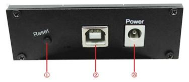
1 It is the reset button, when the controller crash, can touch this key to reset.
