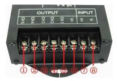
(1) It is the load output 5th channel negative pole;
