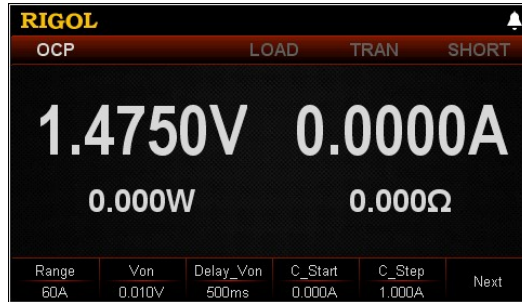
Figure 2-30 Main Interface of OCP Test Function
