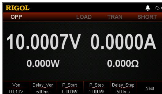
Figure 2-34 Main Interface of OPP Test Function
