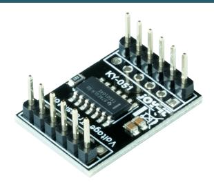
This module converts digital signals from one voltage down to another or up. This makes it possible to operate sensors and modules that work with 5 V logic with 3 V systems, such as the Raspberry Pi, and vice versa.
