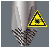
A precisely-focused laser creates a sharp-edged surface structure. This laser treatment results in an edge hardness of up to 1000 HV 0.3. Wera Lasertip "bites" itself into the screw head and prevents any slips out of the recess. It is available for screwdrivers for slotted, Phillips and Pozidriv
