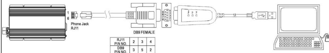
When a MOXA converter is used to achieve connection between inverter and PC, the PC should be powered-on first before inserting the USB end of the MOXA converter, otherwise proper communication link can not be made.
