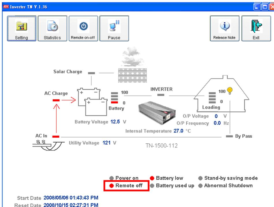
To turn the inverter back ON, click-on the Remote on-off icon, the inverter will come back online after a “beep.” The “Remote off” indication on the monitoring menu will change back to “Remote on” confirming the ON status.
