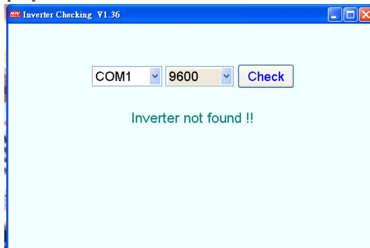
To bypass error: First make sure the COM port setting are the same for both the software and PC/notebook. This can be done by checking the PC' s hardware manager. Also, check for possible loose cable connection.
