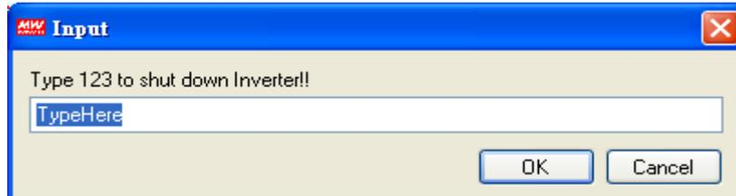
At TypeHere enter “123” then press OK and the inverter will turn OFF after it gives out a “beep.” The Remote ON indication on the monitoring menu will now change to Remote OFF which confirms it’s off status. Refer to the menu below :
