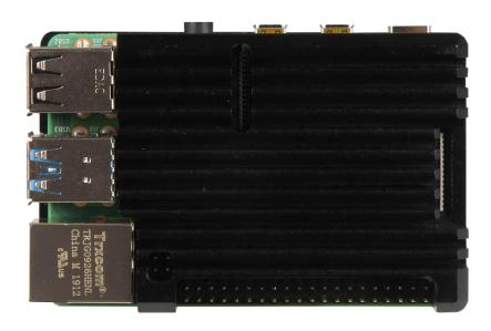
3. Now, turn the Raspberry Pi 4 with the top around, put on the bottom part and screw the case tight at the bottom with the allen key included in the scope of delivery.
