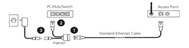
There is an official Power-over-Ethernet standard that allows devices and routers to activate a 48VDC power line on the unused Ethernet pins (4,5 and 7,8) but PoE is expensive, requiring a special router and then a step-down converter to handle the high 48V line.
