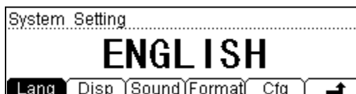
Figure 2-83 The Interface of Setting the System Function
