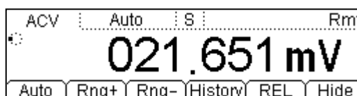
Figure 2-7 AC Voltage Measurement Interface
