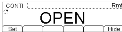
Figure 2-26 Continuity Testing Interface
