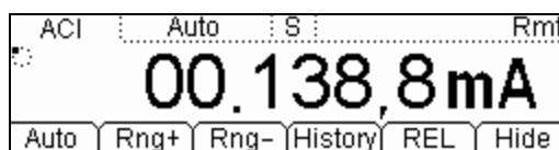
Figure 2-14 AC Current Measurement Interface
