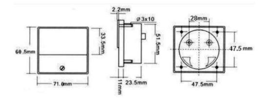
Moving coil panel meters for use in electronic instruments, switchboards, vehicles, with zero adjusting screw. Class 2.5.
