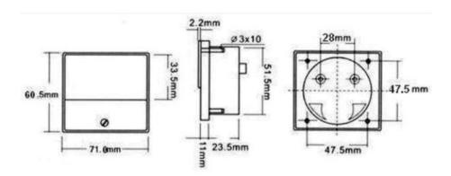
Moving coil panel meters for use in electronic instruments, switchboards, vehicles, with zero adjusting screw. Class 2.5.
