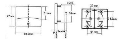
Moving coil panel meters for use in electronic instruments, switchboards, vehicles, with zero adjusting screw. Class 2.5.
